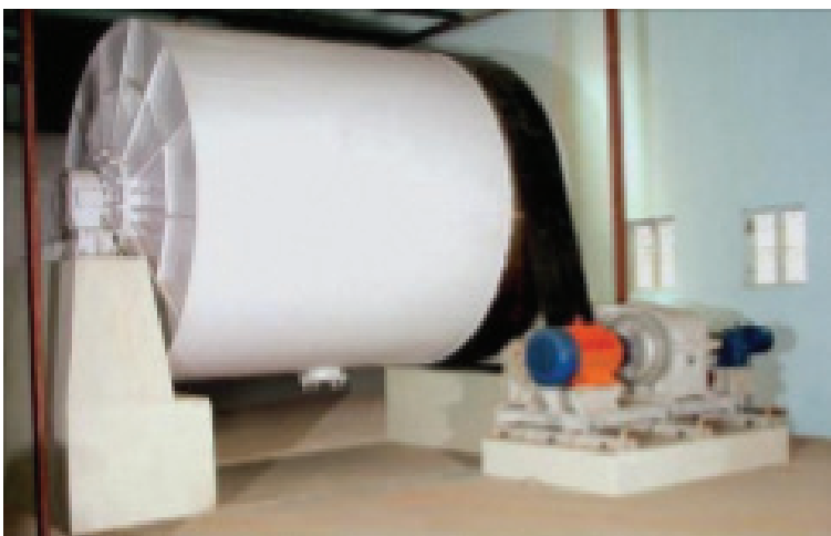
Figure 25: Conventional Ball Mill system
