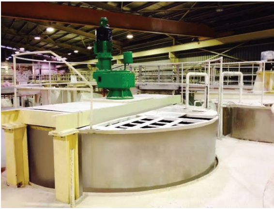
Figure 6: Slip agitation and storage
